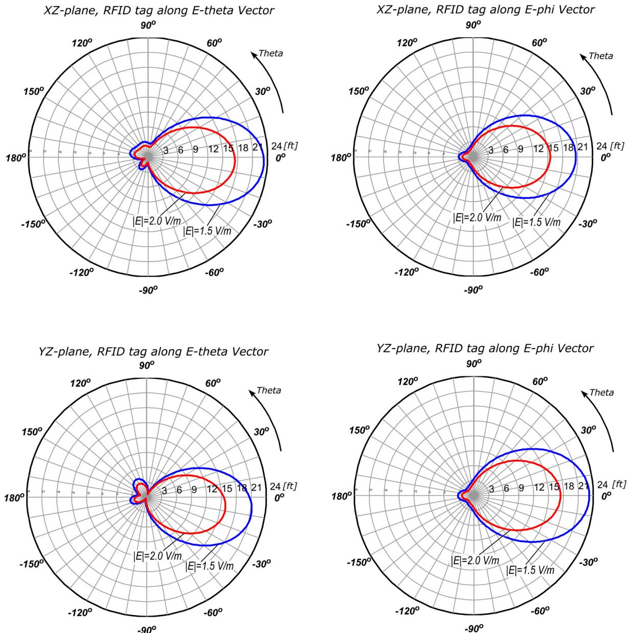
The Read Range Patterns illustrate the reading zones for two tags. One zone is for the tags require the activation field strength 1.5 [V/m]. It corresponds approximately to the Alien Squiggle Inlay "ALN-9540" with Higgs-2 RFID IC or NXP SL3ICS1202. Second zone is for tags require the activation field strength 2.0 [V/m]. It corresponds approximately to the tag with Impinj "Monza-2" RFID IC.
