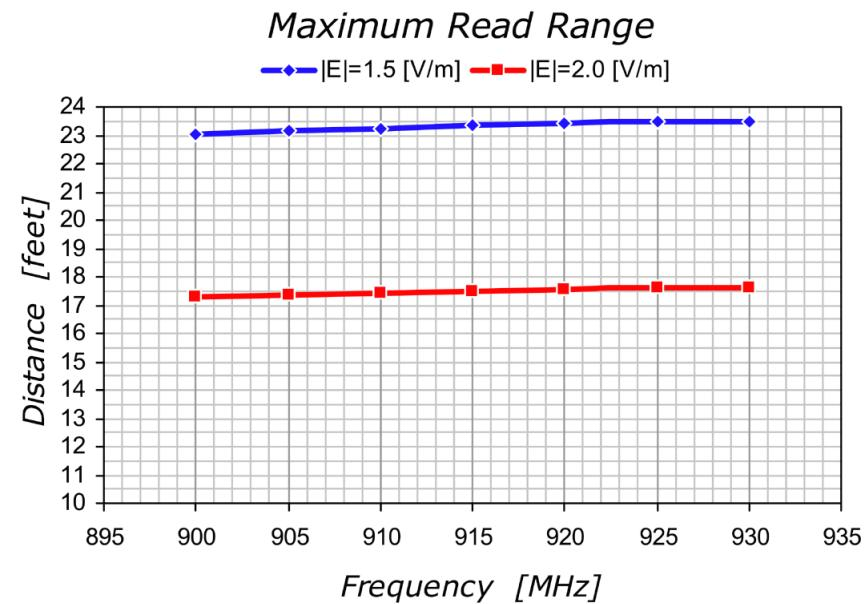
The Blue Curve corresponds to the tags require the activation field strength 1.5 [V/m]. The Red Curve corresponds to the tags require the activation field strength 2.0 [V/m].
