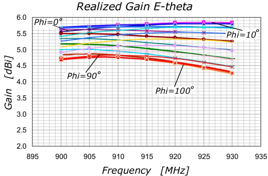
Angle Phi variation is from  $0^\circ$  to  $+180^\circ$ , angle Theta is  $0^\circ$ .
